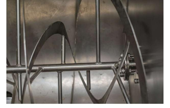
The task in hand was to blend recently milled metal powders – titanium or zirconium - before transfer to a hydraulic press for compaction into disks. In December 2010, one particular batch was never completed. In fact, that batch provided the fuel for a dust fire and explosion, originating inside a *paddle blender*, resulting in the deaths of 3 operators; 2 died at the scene and the 3<sup>rd</sup> died later with severe burn injuries.
